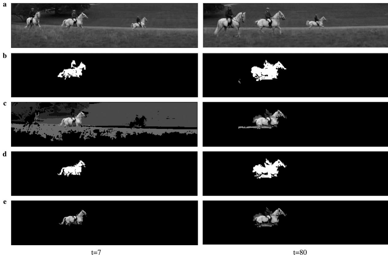
Fig. 16. Sequence of selective attention on one horse in different time instants. (a) Input image. (b) “Active” pixels of the Interest Map. (c) Working Memory. (d) Attention Focus. (e) Attention Focus overlapped with input image.
